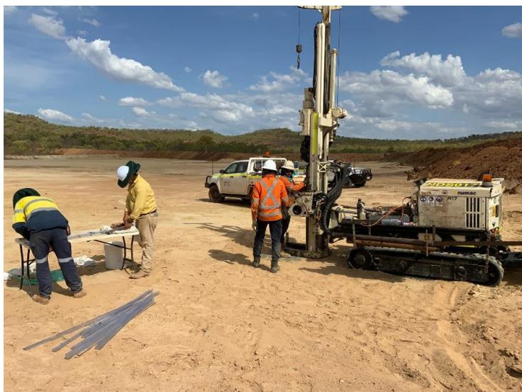
**Figure 1. Push-rod rig onsite at the Tailings Storage Facility.**
