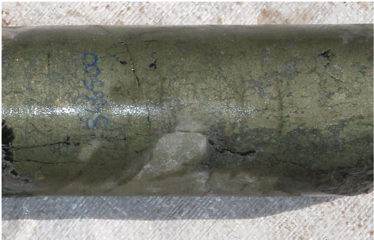
Massive chalcopyrite zone formed within mudstone host, BLDD09-002 at 196m depth.
