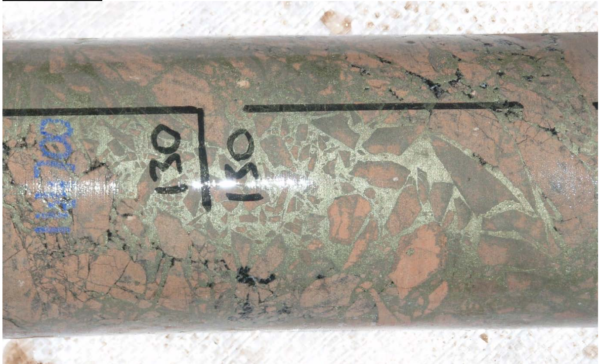
Chalcopyrite matrix infilling brecciated trachyte host, BLDD09-002 at 130m depth.
